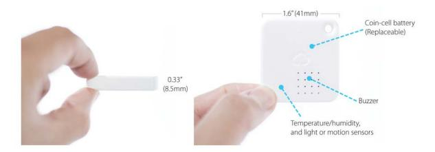
Highly accurate wireless ambient (air) temperature logger allows you to monitor your critical temperatures in near real time with alerts sent direct to your mobile phone.
